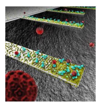
This rendition depicts an array of tiny, diving-boardlike devices called nanocantilevers. The devices are coated with antibodies to capture viruses, which are represented as red spheres. New findings about the behavior of the cantilevers could be crucial in designing a new class of ultra-small sensors for detecting viruses, bacteria and other pathogens. (Image generated by Seyet, LLC)
