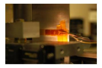
Engineers at Southwest Research Institute have developed new multi-layer thin films and combined them with magnetostrictive sensors to nondestructively detect and monitor defects in aircraft components. The probe and sensor were evaluated on an A-10 aircraft test article and successfully detected a crack and monitored its growth. Unlike MsS methods that evaluate flaws in pipeline, the MsS method for aircraft does not require the use of external magnets. Credit: Southwest Research Institute
