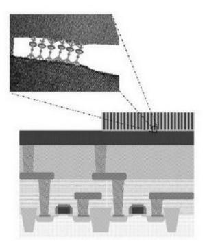
In this cross-section of a portion of the hypothesized hybrid micro-nanomolecular IC, a crossbar (vertical lines) is placed on top of conventional CMOS circuitry. The inset drawing shows the molecules that link the lower and upper sides of the crossbar and "mimic the behavior of a flash memory cell." Photo credit: Cerofolini, G. et al.
