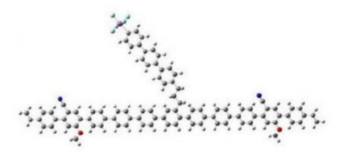
This hypothetical molecule is a candidate for mimicking a flash memory cell. In Cerofolini and Mascolo's design, thousands of molecules are grafted to the silicon structure at each cross point. Photo credit: Cerofolini, G. et al.
