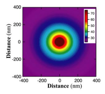
A gold nanobead, trapped with 205 milliwatts of infrared laser light, heats up to about 75 degrees C or 167 degrees F (shown in dark red) and the temperature in the surrounding area gradually cools off (the purple area is about 40 degrees C or 104 degrees F). Credit: Yeonee Seol/JILA
