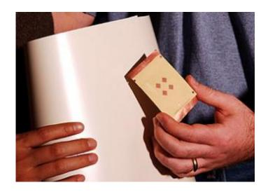
This close-up shows an antenna array embedded on liquid crystal polymer (right). To the left is a large sheet of the flexible, weather-resistant polymer. Georgia Tech Photo: Gary Meek
