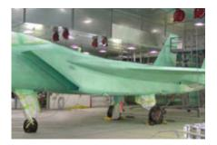
Chrome-free inhibitor technology developed at UMR is being used to coat F-15s. The primer is an aqua green color. The aircraft are later painted gray.
