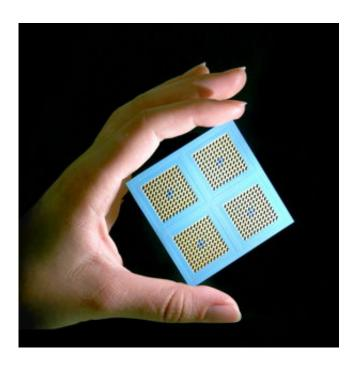
Integrated ceramic micro fuel cell system for portable applications. © Fraunhofer IKTS
