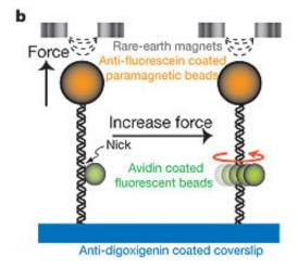
To test what happens when a DNA molecule is overwound, the DNA was stretched between a glass coverslip and a paramagnetic bead, while a fluorescent avidin-coated rotor bead was attached to the DNA just below a biochemical nick. Tension in the DNA was controlled by raising or lowering the magnets, and changes in winding were observed by tracking the rotation of the fluorescent bead.
