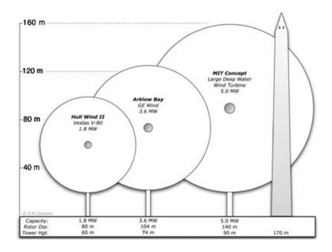
This figure shows (from left to right) an onshore wind turbine, a conventional offshore unit, and the experimental unit used in MIT's concept for a deep-water floating turbine. In each case, the disk indicates the area swept by the turbine blades. The Washington Monument in Washington, DC, appears for comparison. Image courtesy / Stephen Connors, MIT
