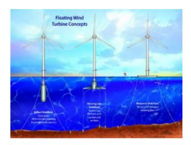
Among three designs for floating giant wind turbines in the deep ocean, MIT research is focusing on the tension leg platform (center), a system that oil companies use for deep-water rigs. Image courtesy / National Renewable Energy Laboratory
