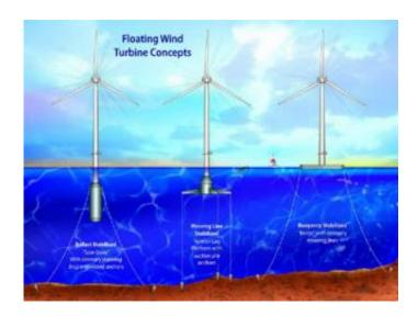
Among three designs for floating giant wind turbines in the deep ocean, MIT research is focusing on the tension leg platform (center), a system that oil companies use for deep-water rigs. Image courtesy / National Renewable Energy Laboratory
