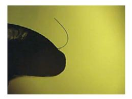
Microscopic flash photography shows a carbon fiber 5 microns in diameter bending nearly 90 degrees while driven to oscillate at 33.4 kHz. The combined flexibility and durability of carbon fibers suggest many uses in microelectromechanical (MEMS) devices, including use as springs and as supports for vibrating objects. Credit: Thompson Lab/Cornell University
