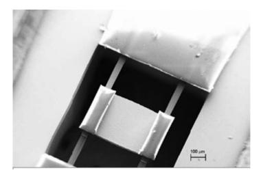
Carbon fiber rods supporting this tiny mirror can be made to bend up to 90 degrees millions of times without showing fatigue. The technology could be used to create a video projector on a chip. Credit: Thompson Lab/Cornell University
