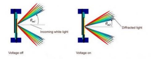
Tunable diffraction grating. The vertical membrane is made of artificial muscle, and has carbon electrodes attached to its sides. The membrane has one side molded into a diffraction grating and coated with gold to increase reflectivity. As the applied voltage varies, so does the periodicity of the diffraction grating, changing the angle of the diffracted light.
