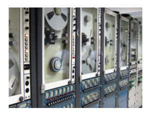
The machines pictured read the 1-inch-wide magnetic data tape from their 14-inch round reels. Multiple machines are used because each reel only records about 15 minutes worth of data. As one reel fills, the next machine automatically starts recording a slight overlap for data continuity. Credit: NASA.
