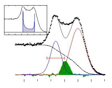
Spectral data from an ARPES study at Beamline 7.0.1 of Berkeley Lab's Advanced Light Source revealed the two discrete peaks (blue for the holon and red for the spinon) that form the signature signal of a spin-charge separation event.
