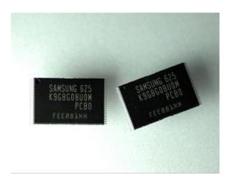
Samsung Electronics today announced that it has begun mass producing an 8-Gigabit (Gb) NAND flash memory device, providing a much larger and more affordable storage density for consumer and mobile applications such as mobile phones, MP3 players and gaming consoles. The high-density MLC (multi-level-cell) memory is being produced with 60-nanometer process technology - the smallest used today.
