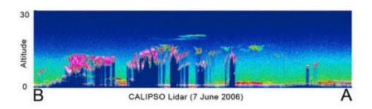
A lidar profile from the CALIPSO spacecraft, specifically the 523 nanometer Total Attenuated Backscatter. To view a higher resolution version with altitude information and latitude and longitude of the gathered data, click on the image. Credit: NASA Langley Research Center.
