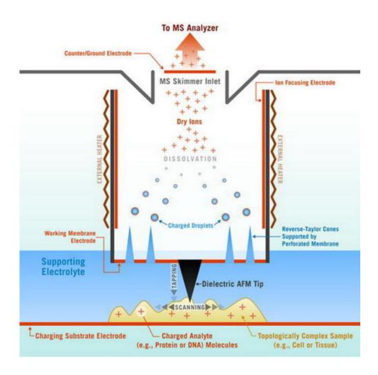
Georgia Tech&acutes SMS Probe gently pulls biomolecules precisely at a specific point on the cell/tissue surface, ionizes these biomolecules and produces "dry" ions suitable for analysis and then transports those ions to the mass spectrometer.
