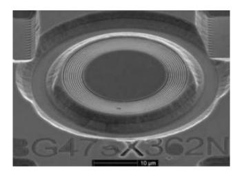
Etched nanostructured rings around an LED can make it more than seven times brighter. The novel technique developed at NIST may have applications in areas such as in biomedical imaging where LED brightness is crucial. Credit: NIST
