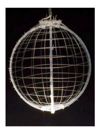
A sphere-shaped web of photo-detecting fibers developed by MIT scientists can sense the optical properties of the entire volume of space around it, as well as detect the source of incoming light. Image courtesy / Greg Hren
