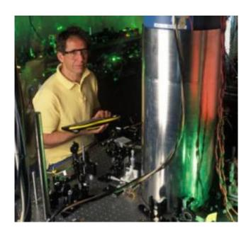
NIST physicist Jim Bergquist holds a portable keyboard used to set up the world's most accurate clock. The silver cylinder in the foreground is a magnetic shield that surrounds a cryogenic vacuum system, which in turn holds the heart of the clock, a single mercury ion (electrically charged atom). The ion is brought to rest by laser-cooling it to near absolute zero. Credit: ©Geoffrey Wheeler
