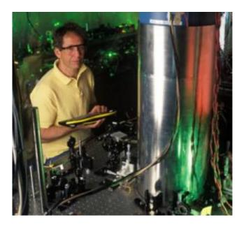
NIST physicist Jim Bergquist holds a portable keyboard used to set up the world's most accurate clock. The silver cylinder in the foreground is a magnetic shield that surrounds a cryogenic vacuum system, which in turn holds the heart of the clock, a single mercury ion (electrically charged atom). The ion is brought to rest by laser-cooling it to near absolute zero. Credit: ©Geoffrey Wheeler
