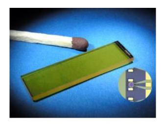
Polymer chip with a micro-spectrometer: Indium phosphite photodiodes are integrated on this polytronic chip with its tiny circuit paths made of plastic. © Fraunhofer HHI
