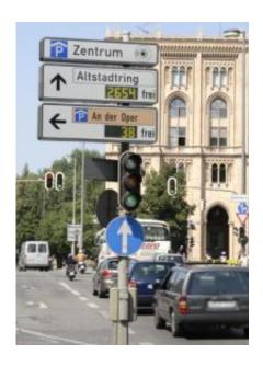
The world's first parking guidance system to dispense with wires and underground connections turned in a stellar performance during its first 100 days of operation. In service in Munich (Germany), the system uses GPRS transmission to transfer data and control signals among all of the inner city's 25 parking garages.
