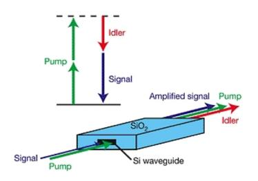
In four-wave mixing, two photons at a pump wavelength are converted into two new photons, one at the signal wavelength and one at a wavelength equal to twice the pump wavelength minus the signal wavelength. The new signal photons combine with the originals to create an amplified signal. The idler photons are a copy of the signal at a new wavelength, so the system can be used to convert a signal from one communications channel to another. Credit: Gaeta Group/Cornell University
