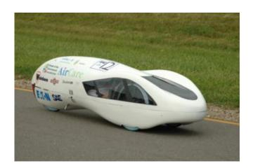
"We achieved this level of efficiency by optimizing many aspects of the vehicle design, including: aerodynamics, light-weight construction, a small displacement engine (54 cc), and conservative driving habits," says Team Captain Kevin Li.
