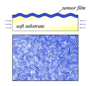
NIST researchers developed a new high-speed method for measuring the stiffness of soft-polymer materials like those used in contact lenses. The test material is covered with a sensor film, and the combination is compressed until it buckles. The resulting pattern of ridges is the key to determining stiffness, an important material property. Credit: NIST
