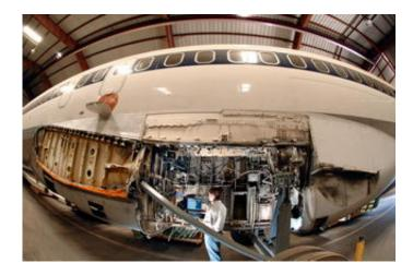
Sandian Kevin Howard inspects electrical wiring in the wheel well of a retired Boeing 727 at Sandia's FAA Airworthiness Assurance NDI Validation Center. The wing on the 727 has been removed. (Photo by Randy Montoya)
