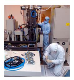
Vistec Semiconductor Systems technicians John Cunanan, (standing) a field simulation engineer, and Paul Whitwood, a final test engineer, conduct tests on a Leica Vector Beam photolithography machine in the cleanroom at the Birck Nanotechnology Center's Scifres Nanofabrication Laboratory. The \$6 million instrument will help Purdue nanotechnology researchers write on computer chips ultra-high resolution lines that are as small as 6 nanometers. Photo: David Umberger
