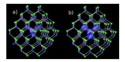
In an example of doped nanocrystals, this charge density plot shows magnesium impurities in cadmium-selenium nanocrystals at two different gap levels: (a) resonant and (b) hybrid. Image credit: Gustavo Dalpian and James Chelikowsky.
