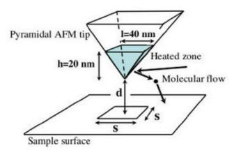
In this drawing of an atomic force microscope tip transferring heat to a surface, the heated zone causes air molecules to collide, which heats a specific, localized surface with no contact. The technique could help develop heat-assisted magnetic recording, an innovative alternative for future data storage technology. Photo credit: Pierre-Olivier Chapuis et al.
