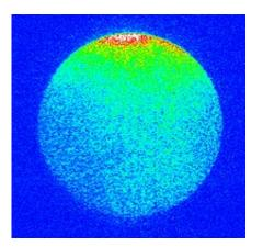
Argonne engineers are the first to capture hydrogen combustion images inside an engine operating at real-world speeds. The red and yellow images show the more intense temperatures.
