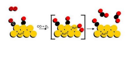
Mechanism for the catalytic reaction 2CO + O2 -> 2CO2
