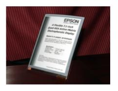
Seiko Epson Corp. has successfully developed A6-size (7.1 inches on the diagonal) electronic paper using a plastic substrate. Drawing on Epson's original SUFTLA technology, the new electronic paper achieves Quad-XGA resolution (1536 x 2048 pixels) – the world's highest – and shows the potential for increasing screen size. The development was announced on June 9 at the Society for Information Display (SID) international symposium held in San Francisco.
