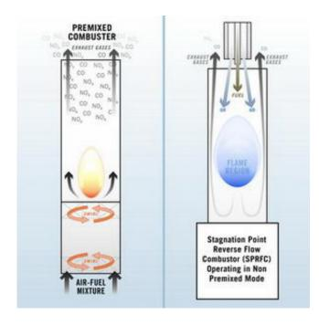
A comparison of Georgia Tech's combustor with a traditional combustor: (Left) A traditional combustor mixes fuel and air before they are injected into the combustion chamber. (Right) Tech's combustor injects the fuel and air separately into the combustor.
