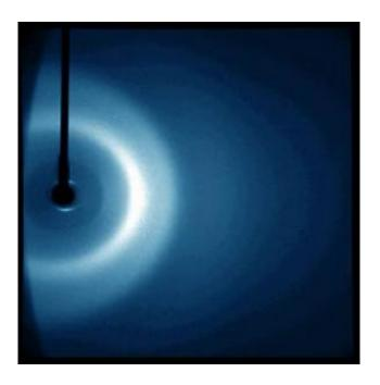
X-ray scattering pattern of liquid water at room temperature and pressure obtained at Beamline 7.3.3 of the Advanced Light Source at the the Lawrence Berkeley National Laboratory. Credit: Lawrence Berkeley National Laboratory
