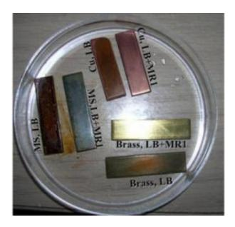
Brass, mild steel (MS) and copper (Cu) samples compared after incubation with (+MR1) and without the presence of the bacteria. Credit: Corrosion and Environmental Effects laboratory, Mork Family Department of Materials Science and Chemical Engineering, Viterbi School of Engineering
