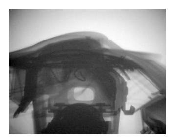
Airbag ignition with subsequent unfolding and cover release. X-ray cinematography images of two selected moments in the sequence. © Fraunhofer EMI
