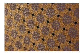
Connecting antenna elements in a revolutionary way could allow a new ultrawideband antenna to replace as many as five conventional antennas. Georgia Tech Photo: Gary Meek
