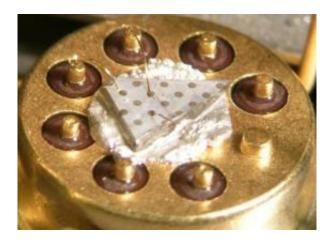
This is a close-up image of a tiny hydrogen sensor developed by University of Florida engineering researchers. The sensor uses extremely small zinc oxide nanorods, located within the black dots in the triangular base, to gauge the amount of hydrogen in the air. To power the sensor, the researchers designed a novel device that harvests energy from vibrations where the sensor is placed. A tiny wireless transmitter enables the sensor to transmit its results to a central base station.
