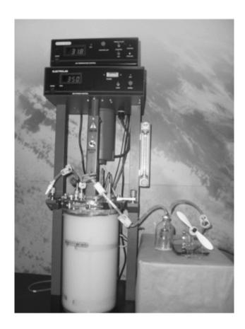
Coupling of Bio-H<sub>2</sub> made by fermentation of confectionery waste to the operation of a PEM fuel cell used to drive an electrical device.
