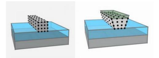
The silicon waveguide at left contains a crystal symmetry and no electro-optic effect. At right, the silicon waveguide has a straining layer that breaks the symmetry. The broken symmetry makes it possible to change the phase of light by applying an electric field across the waveguide, which can create an electro-optic modulator. Photo credit: Rune Jacobesen.
