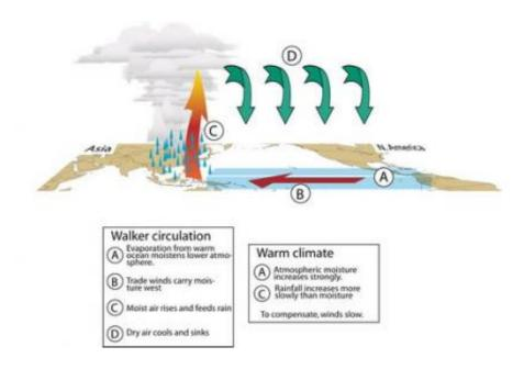
This diagram shows the Walker Circulation, a vast loop of air above the equatorial Pacific ocean. Courtesy Gabriel Vecchi, UCAR.
