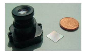
Scientists fabricated an artificial apposition compound eye (center) that is significantly cheaper and smaller than a traditional 20-mm single lens objective (left) with the same magnification; and much smaller – though not quite as cheap – as a Euro cent (right). Photo credit: IOP.
