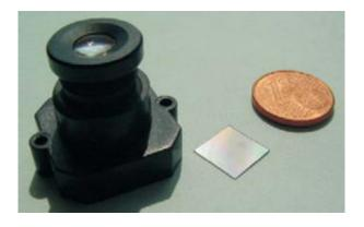
Scientists fabricated an artificial apposition compound eye (center) that is significantly cheaper and smaller than a traditional 20-mm single lens objective (left) with the same magnification; and much smaller – though not quite as cheap – as a Euro cent (right). Photo credit: IOP.
