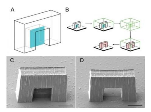
Replication of a master structure with a closed loop. The drawings above depict the master structure for the creation of an arch. The blue plane is the membrane. (C) is a master structure for the arch. (D) is the corresponding daughter structure. The Fourkas group.
