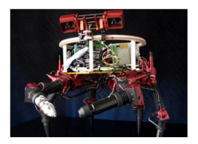
The crawling robot, Lemur, was built to help astronauts complete small jobs in space. "Lemur could be an astronauts pet monkey," says JPL engineer Brett Kennedy who designed the 6-limbed robot. Lemur performs a variety of functions with attachable tools.
