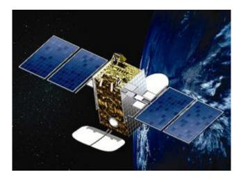
HYLAS is a hybrid Ka Band/Ku Band satellite with European coverage. The satellite will be used mainly to provide broadband Internet access and to distribute and broadcast High Definition Television (HDTV). Credits: Avanti
