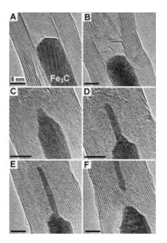
An iron carbide nanowire is squeezed through the center of a multi-walled carbon nanotube. Credit: Johannes Gutenberg University/Banhart
