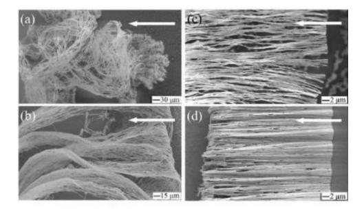
This series of scanning electron microscope images shows how increasing an electric field can align a bundle of silver nanowires, from disordered (a) to highly aligned (d). The white arrow indicates the direction of the electric current, which caused silver ions to migrate in the opposite direction. Credit: Jialin Sun
