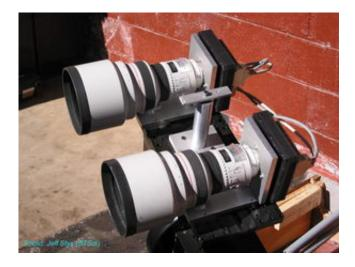
Astronomers used this inexpensive telescope to find an extrasolar planet transiting the face of a Sun-like star 600 light-years from Earth. The telescope, which looks like a pair of binoculars, consists of two 200-millimeter telephoto camera lenses. The lenses are attached to electronic devices that measured slight dips in light output from the star, indicating that an object was crossing in front of it. The telescope is on the summit of the Haleakala volcano in Hawaii. Credit: NASA
