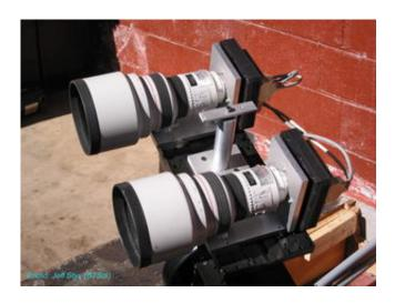
Astronomers used this inexpensive telescope to find an extrasolar planet transiting the face of a Sun-like star 600 light-years from Earth. The telescope, which looks like a pair of binoculars, consists of two 200-millimeter telephoto camera lenses. The lenses are attached to electronic devices that measured slight dips in light output from the star, indicating that an object was crossing in front of it. The telescope is on the summit of the Haleakala volcano in Hawaii. Credit: NASA
