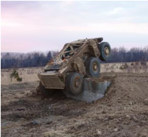
Crusher can climb > 4 foot steps
