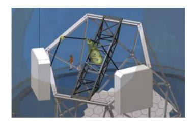
This computer rendering shows what the upgraded prime focus package on the Hobby-Eberly Telescope will look like, as well as the location of new spectrographs, both critical parts of the Hobby-Eberly Telescope Dark Energy Experiment (HETDEX). Image: HETDEX Team/McDonald Observatory
