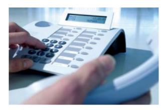
Siemens has developed a telephone system that doesn't require a switchboard. The HiPath BizIP telephones are directly connected to one another and communicate much like participants in an Internet file-sharing service (peer-to-peer, P2P), where computers exchange data without detours through a central server. Designed for up to 16 telephones, the solution is intended primarily for small companies and will make costly installations and maintenance work on telephone systems a thing of the past.
