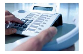
Siemens has developed a telephone system that doesn't require a switchboard. The HiPath BizIP telephones are directly connected to one another and communicate much like participants in an Internet file-sharing service (peer-to-peer, P2P), where computers exchange data without detours through a central server. Designed for up to 16 telephones, the solution is intended primarily for small companies and will make costly installations and maintenance work on telephone systems a thing of the past.
